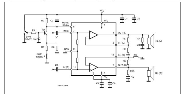
Figure 3. Test and Application Circuit (Stereo Configuration)
